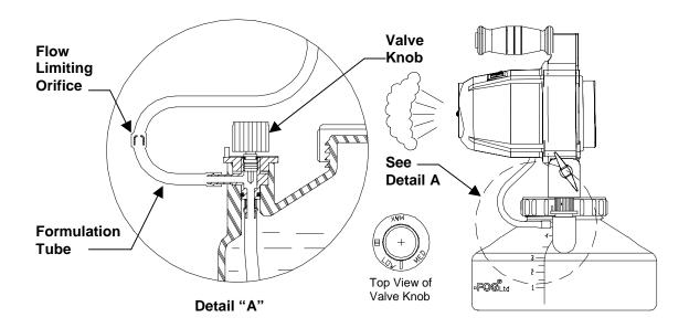
Under normal conditions, the flow rate of the machine, with the valve knob open, is indicated as following:
